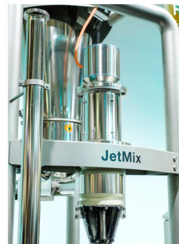
The AKMH stainless steel motors are connected by just one cable, including recirculation to the AKD servo controller. The stainless steel motors can be conveniently designed for different rotational speeds due to their wide adjustment range.
